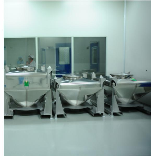
The IBC Blending module enables the mixing of any recipe, at any time.
